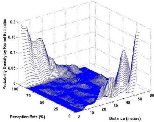
Fig. 3. PDF for distance versus reception rate.
