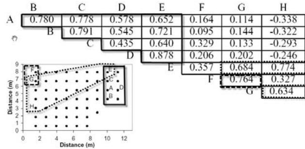
Fig. 10. Covariance Matrix and Layout for Indoor Experiments.
