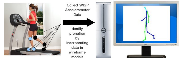
Figure 3. Demo Illustration: WISP sensors will be attached to the runner's leg and feet. Data from the sensor will be used to visualize pronation using a computerized pronation model (Note: Stick Figure from http://www-anw.cs.umass.edu/mtr/research/biped/ ).
